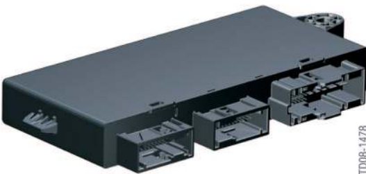
132 - Car Access System control unit
