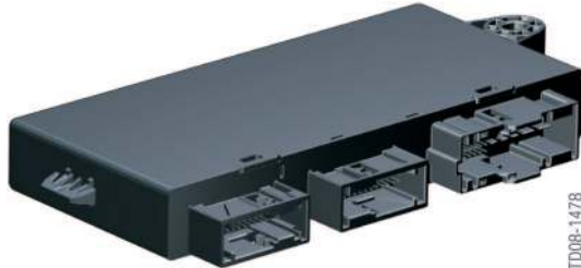
133 - Car Access System control unit
