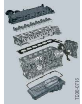
The engine mechanical systems can essentially be divided into the three subassemblies, engine casing components, crankshaft drive system and valvegear. Those three subassemblies are closely interlinked and have to be matched to one another.
