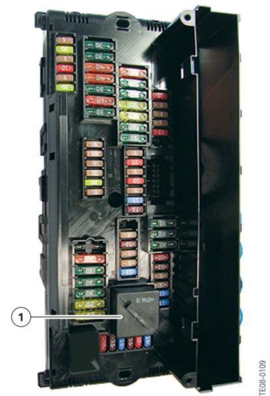
128 - Front fuse board on F01/F02
