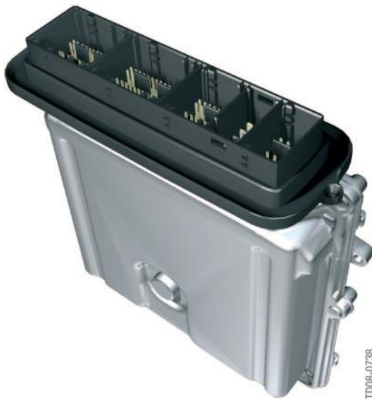
99 - DDE control unit
