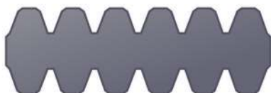
33 - Cross section of a double-sided poly-V-belt
