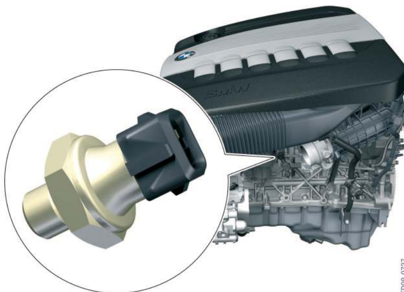
44 - Oil pressure switch location N57 engine
