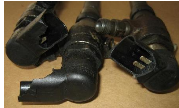
CR Injectors with broken connector housings cannot be repaired
