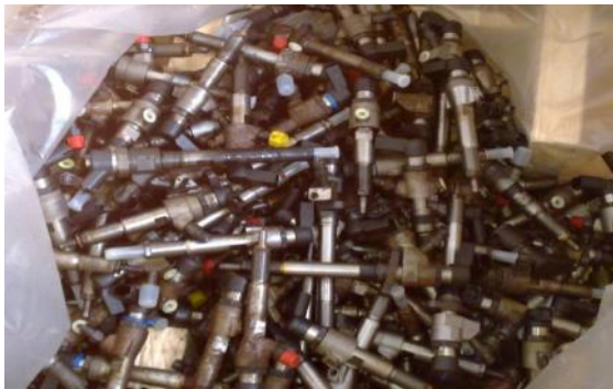
Inappropriate storage can lead to irreparable damages
